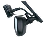
9 - Tighten the stand off with a 3/8" open end wrench. Do not overtighten as the stand off is aluminun and excessive force on the mirror should be avoided. After the appropriate bends have been made to the angle bracket, attach it to the standoff using the supplied button head screw. Make sure there is at least 1\8" clearance between the mirror and any part of the mount.
